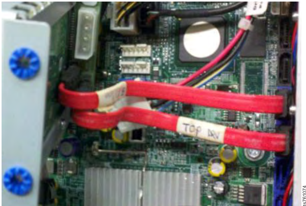
Figure 46. The SATA cables are connected to both the backplane board and the sysplanar.
