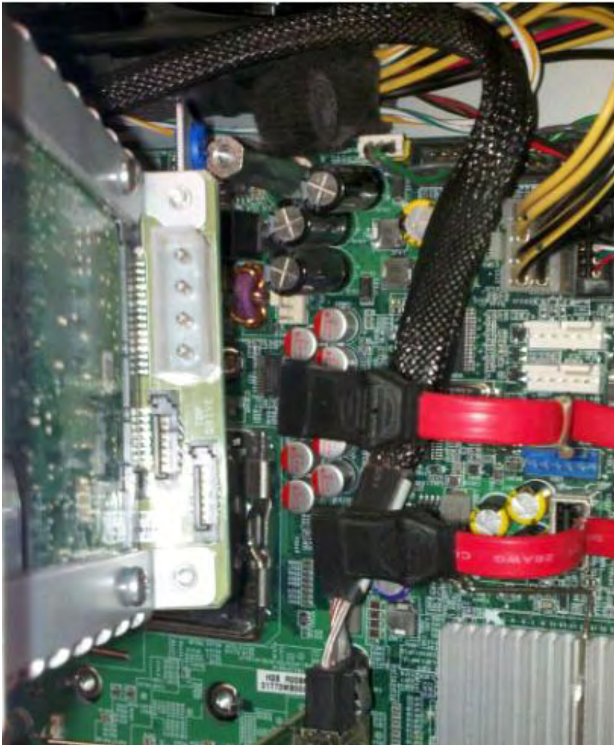
Figure 47. The SATA cables are disconnected from the backplane board.
